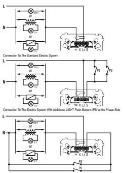
Connection To The Electric System With Additional Light Push-Buttons /PS/ at the Zero Side
