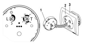
Remove the control unit /1/ and set L knob in the middle position,
