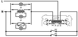
Connection To The Electric System With Additional Light Push-Buttons /PS/ at the Zero Side
