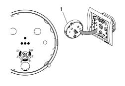
Remove the button /1/ and, using a knob, set the required lighting time up, following the description at the back of the button.
