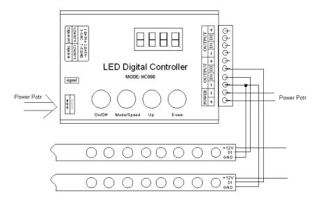
2. Application synchronization (Each controller can be individually powered, can also share power)
